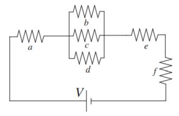
All six resistors in the circuit have the same resistance, R, and the battery is a source of constant voltage, V.
